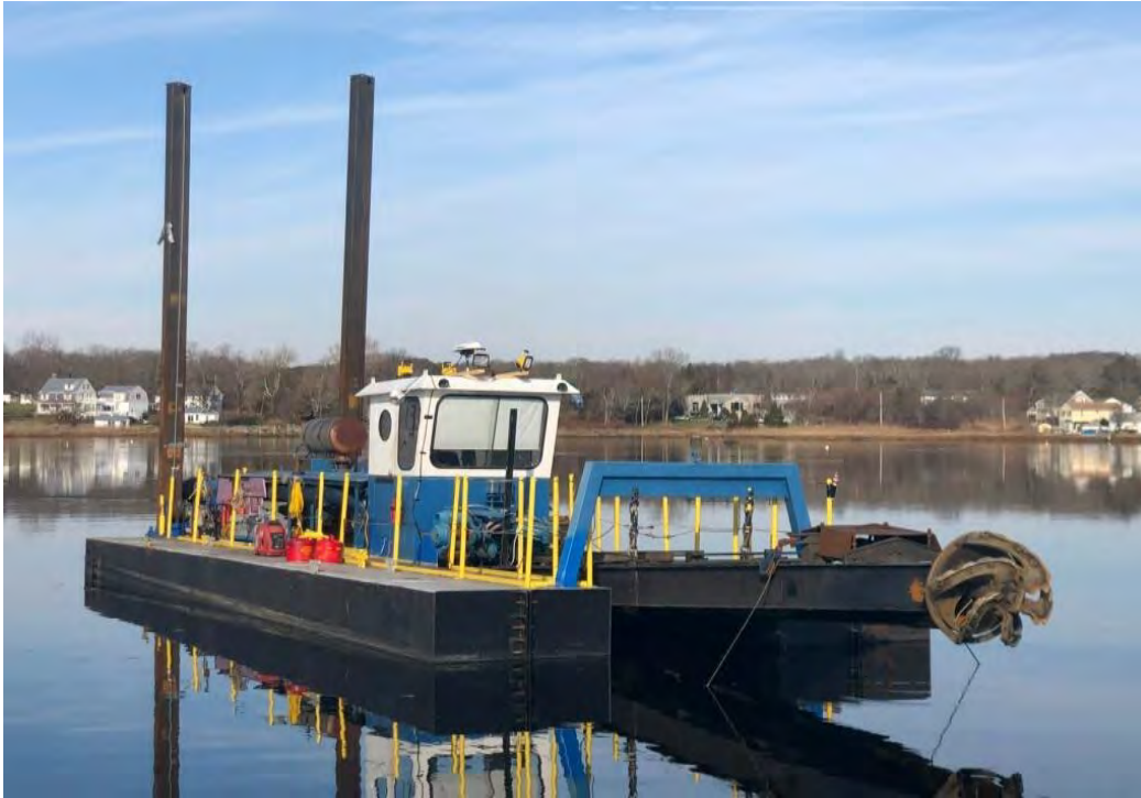
Photo: 2020 Hydraulic Dredge Plant, Oyster Channel, VA.
